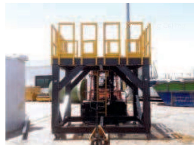
GRP Non conductive mobile maintenance platform
