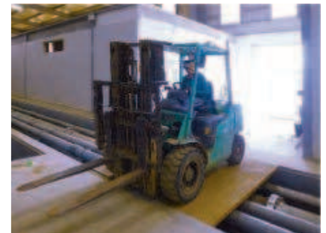
testing Pultruded grating with 3T forklift
